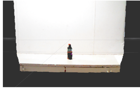
Fig. 7. Front view of the estimated center point of the Iced Tea bottle (seen in pink) from a point cloud 3D perspective.
