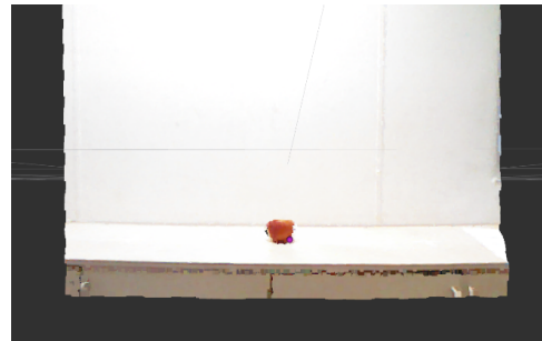
Fig. 9. Front view of the estimated center point of the apple (seen in pink) from a point cloud 3D perspective.
