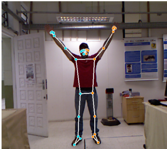
Fig. 5. MediaPipe Pose detecting the person's skeleton with ROS.
