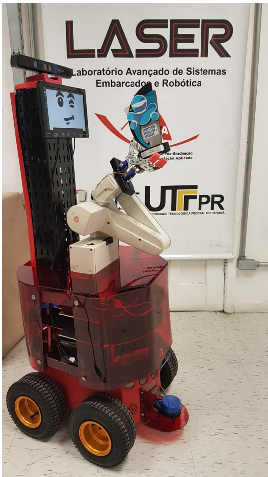
Fig. 1. Side view of the robot subsystems mounted on top of the Pioneer 3-AT base.
