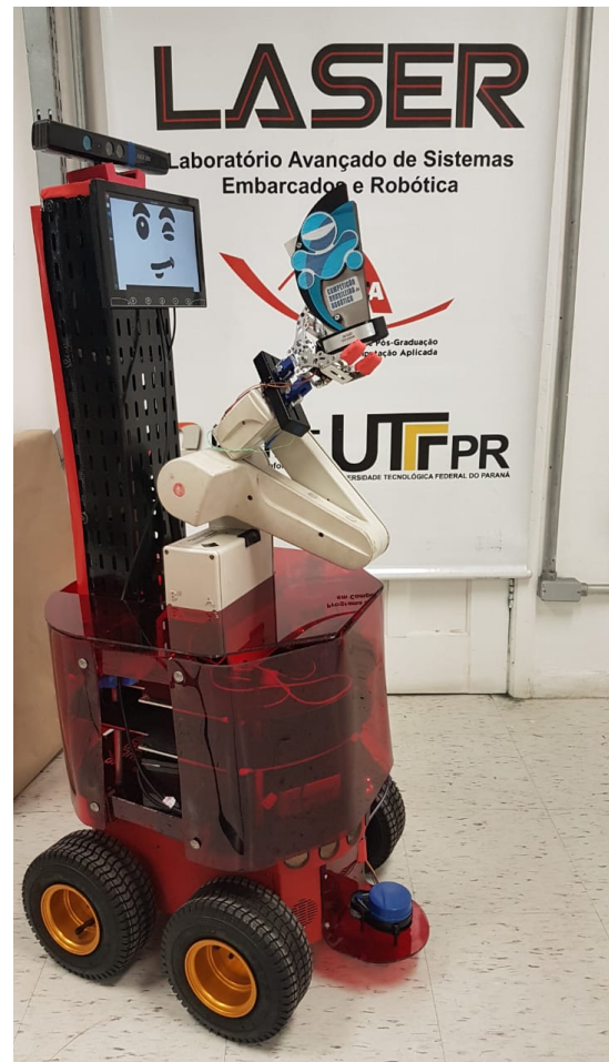
Fig. 2. Side view of the robot subsystems mounted on top of the Pioneer 3-AT base.
