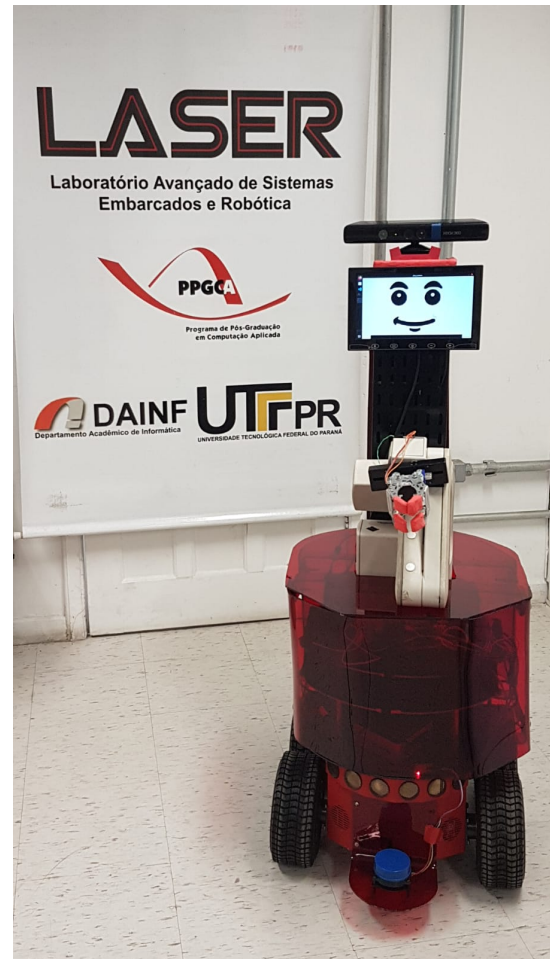
Fig. 1. “Apollo”, composed of a Pioneer 3-AT mobile base, with its sensors (LiDAR, Kinect), the LCD display for simulated emotions, and the manipulator.
