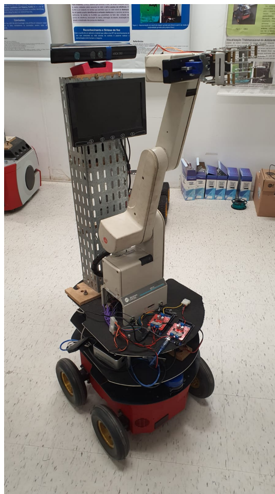
Fig. 1. “Apollo” with its support for the Kinect sensor, the LCD display for simulated emotions and the manipulator.
