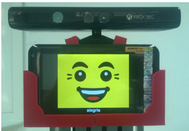
Fig. 4. Simulated emotion presented on the face of the robot.
