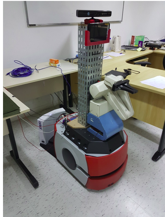
Fig. 2. The manipulation arm mounted in another robot. The plan is to add this manipulator to the Pioneer 3-AT.
