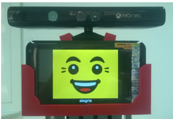
Fig. 4. Simulated emotion presented on the tablet (face) of the robot.
