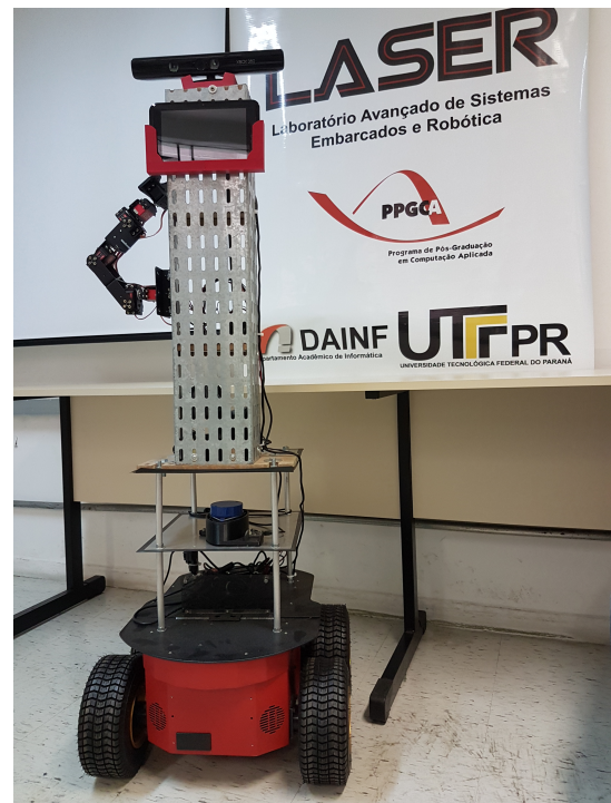
Fig. 1. Pioneer AT (a.k.a. “Apollo”) with its support for the Kinect sensor, and the tablet that is used to present simulated emotions.
