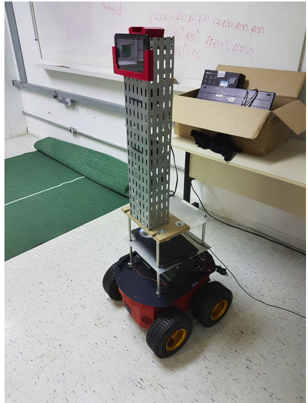
Fig. 2. Pioneer AT (aka "Apollo") with its support for the kinect sensor, and the tablet that is used to present simulated emotions.
