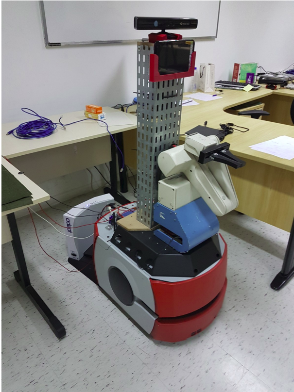
Fig. 1. Pioneer LX (aka "Z") with its articulated arm, kinect sensor and the tablet that is used to present simulated emotions.
