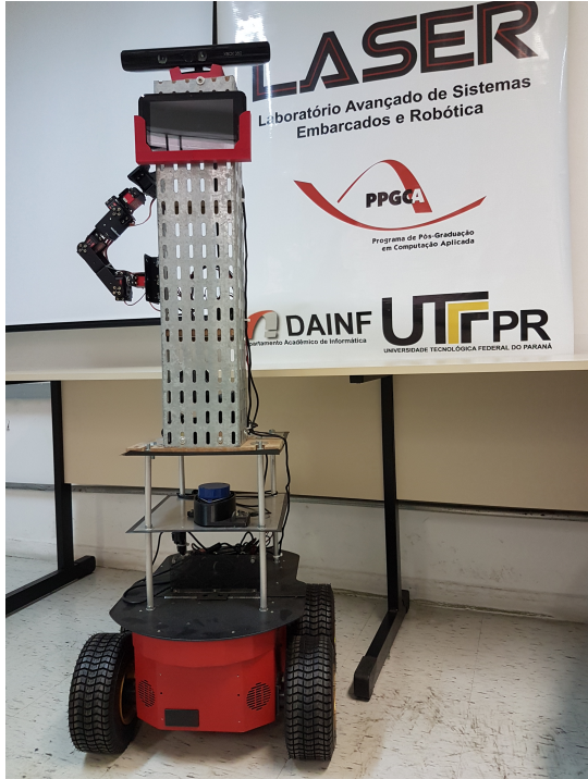
Fig. 2. Pioneer AT (a.k.a. “Apollo”) with its support for the Kinect sensor, and the tablet that is used to present simulated emotions.
