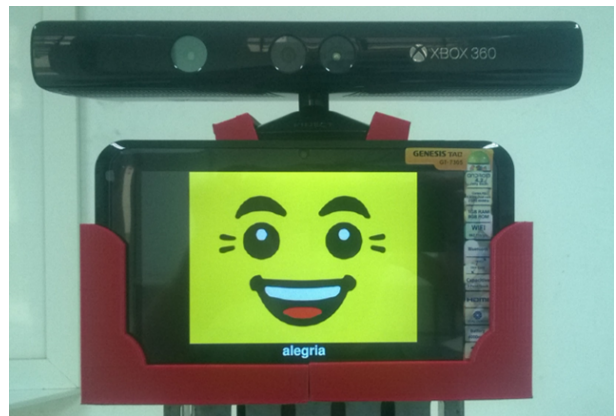
Fig. 3. Simulated emotion presented on the tablet (face) of the robots.
