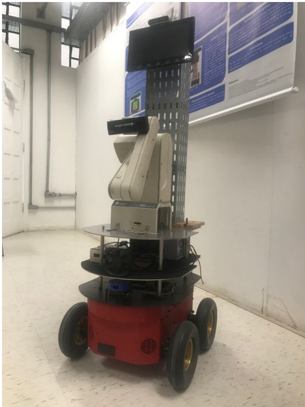
Fig. 1. Pioneer AT (a.k.a. "Apollo") with its support for the RealSense sensor, and the display that is used to present simulated emotions.
